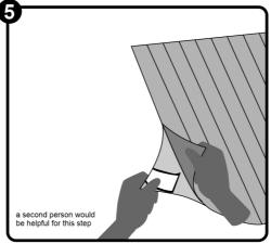
Wet your fingers with the prepared water from the spray bottle and peel off the backing film using the attached sticker.
