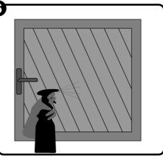
Spray the film again, align, press down with the squeegee and remove bubbles towards the edge (from top to bottom in the middle and to the sides first on the right then on the left, repeat several times)
