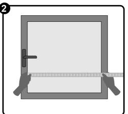
Measure the window area (only glass surface, without rubber seal).
