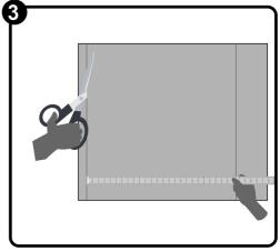
Transfer the dimensions to the carrier film and cut with scissors or a cutter.
