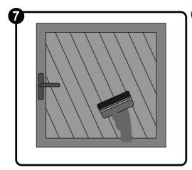
Carefully cut off the overhanging film at the edge with a cutter knife or film cutter so that the window or the rubber is not damaged.
