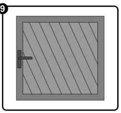
Allow the film to dry for 1-2 days and wait 1 week before cleaning the window in the usual way.
